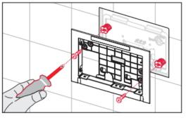
3. Dislodge plate with flat head screwdriver and screw fixing plate to the fixing rods.
