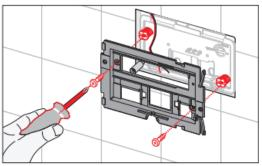
1. Wind the fixing bolts back to 15mm from the finished wall lining and then fit fixing plate.
