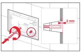
2. Snap rod at point B and wind rod in so that it extends 2mm from the external wall lining.
