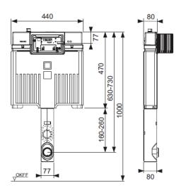
Octa II cistern including "easy fit" flush plate installation for floor standing toilet; depth 8 cm; for installation in or in front of a solid wall.
